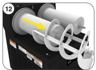
12. Pull Auger from Cooling Drum.
