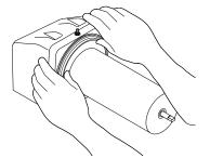
1. Install the seal(s) over the flange at the rear of the cooling drum(s) and press the seal(s) firmly into place as shown.
